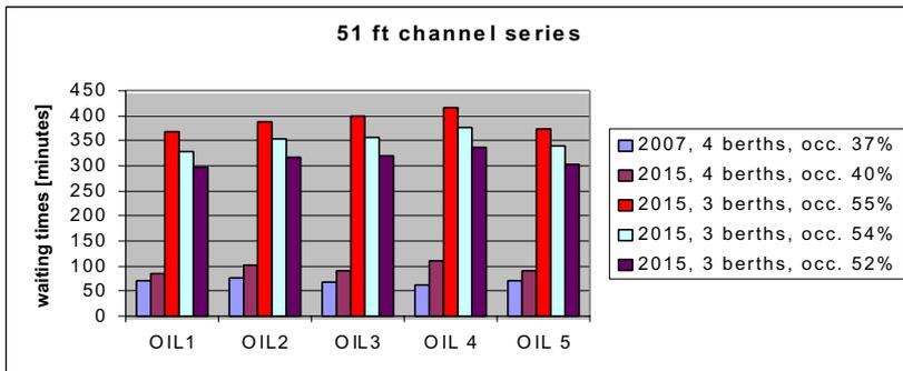
Figure 16. Simulation runs 51-ft channel, oil carriers
