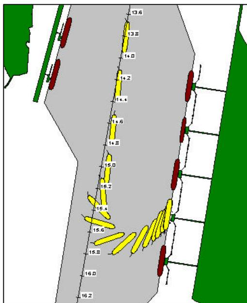
*Figure 10. Track plot of tanker arrival in deep water port*
